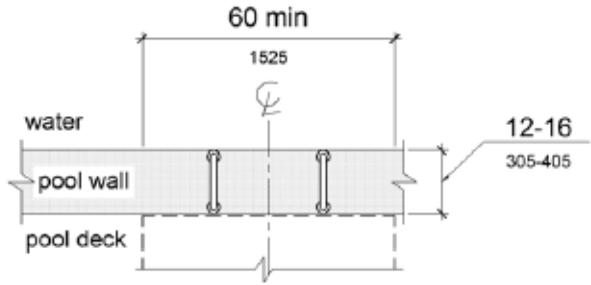
**Figure 1009.4.3 Depth and Length of Transfer Walls**
