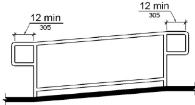
**Figure 505.10.1 Top and Bottom Handrail Extension at Ramps**
