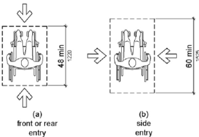
**Figure 802.1.3 Depth of Wheelchair Spaces in Assembly Areas**
