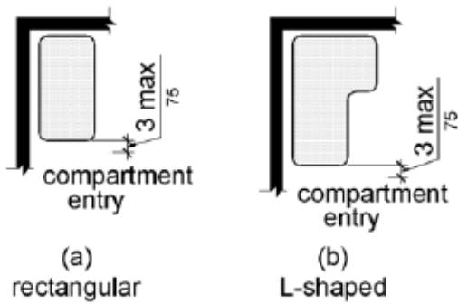
**610.3.1 Rectangular Seats.** The rear edge of a rectangular seat shall be 2 1/2 inches (64 mm) maximum and the front edge 15 inches (380 mm) minimum and 16 inches (405 mm) maximum from the seat wall. The side edge of the seat shall be 1 1/2 inches (38 mm) maximum from the adjacent wall.
