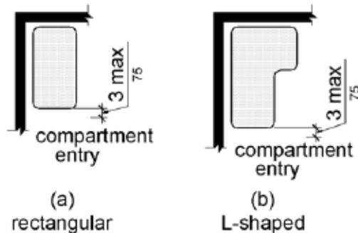
**610.3.1 Rectangular Seats.** The rear edge of a rectangular seat shall be 2 1/2 inches (64 mm) maximum and the front edge 15 inches (380 mm) minimum and 16 inches (405 mm) maximum from the seat wall. The side edge of the seat shall be 1 1/2 inches (38 mm) maximum from the adjacent wall.
