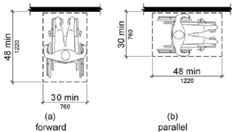
**Figure 305.5 Position of Clear Floor or Ground Space**
