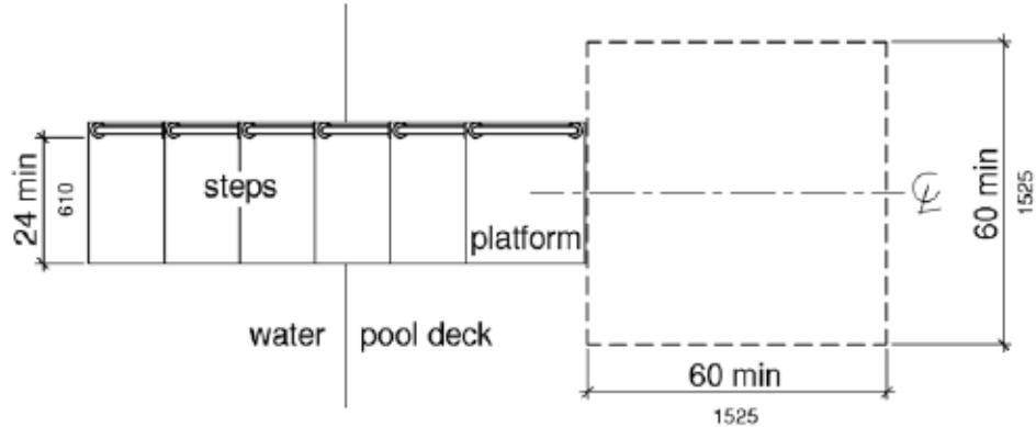
**Figure 1009.5.2 Clear Deck Space at Transfer Platform**
