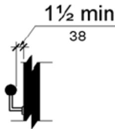
**Figure 505.5 Handrail Clearance**
