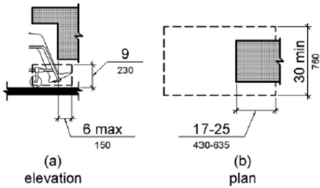
**Figure 306.2 Toe Clearance**
