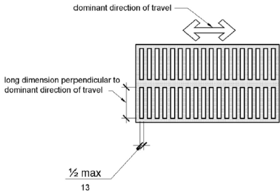
**Figure 302.3 Elongated Openings in Floor or Ground Surfaces**
