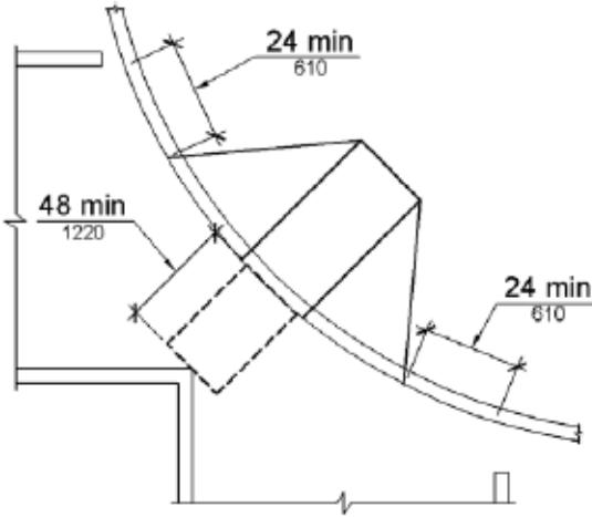
**Figure 406.6 Diagonal or Corner Type Curb Ramps**
