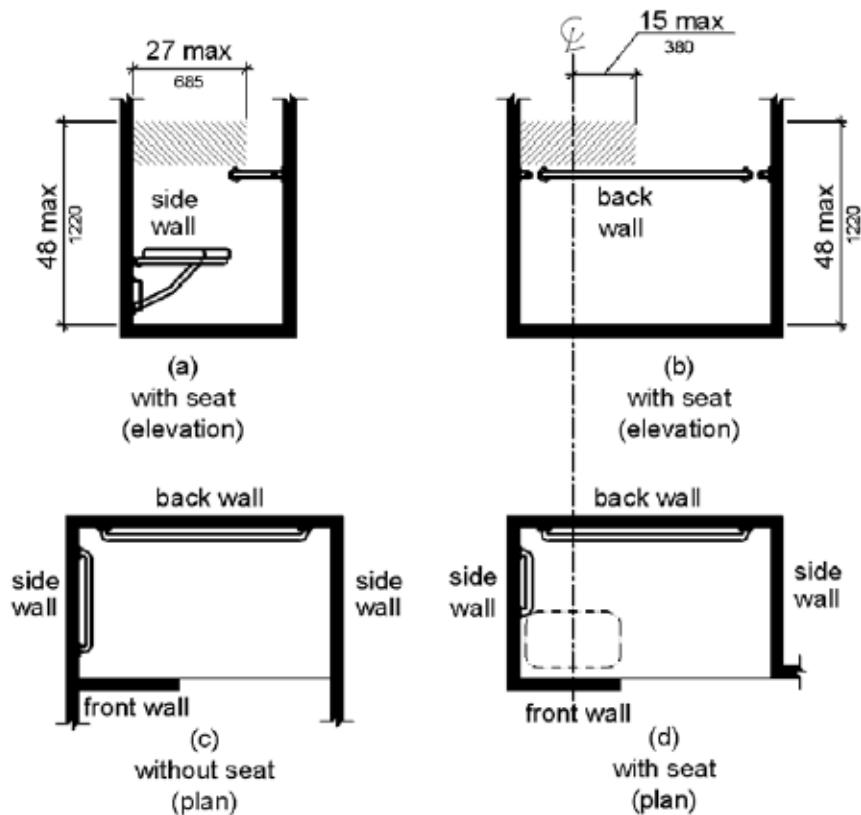
**Figure 608.5.3 Alternate Roll-In Type Shower Compartment Control Location**
