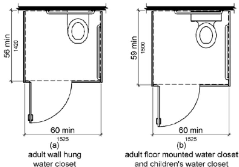
**Figure 604.8.1.1 Size of Wheelchair Accessible Toilet Compartment**
