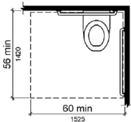
**Figure 604.3.1 Size of Clearance at Water Closets**
