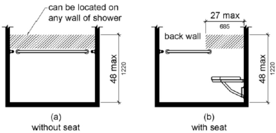
**Figure 608.5.2 Standard Roll-In Type Shower Compartment Control Location**
