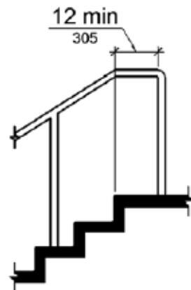
**Figure 505.10.2 Top Handrail Extension at Stairs**
