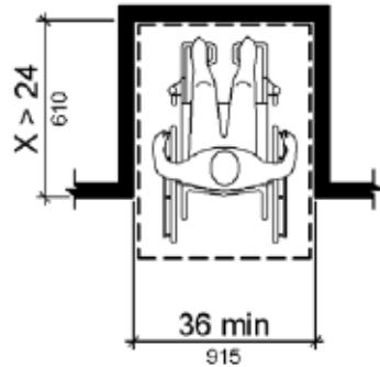
**Figure 305.7.1 Maneuvering Clearance in an Alcove, Forward Approach**
