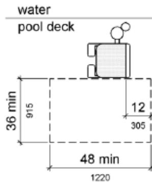
**Figure 1009.2.3 Clear Deck Space at Pool Lifts**
