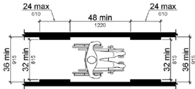
**Figure 403.5.1 Clear Width of an Accessible Route**
