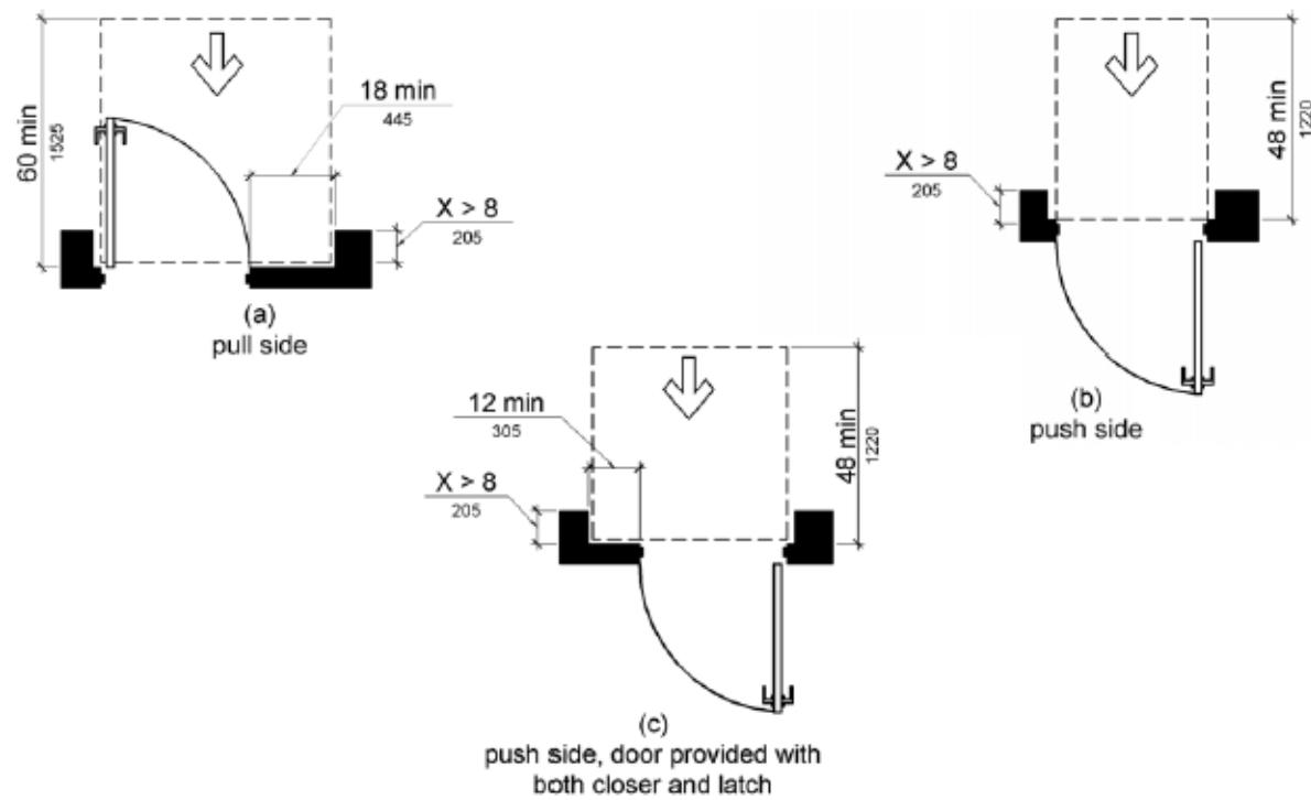
**Figure 404.2.4.3 Maneuvering Clearances at Recessed Doors and Gates**
