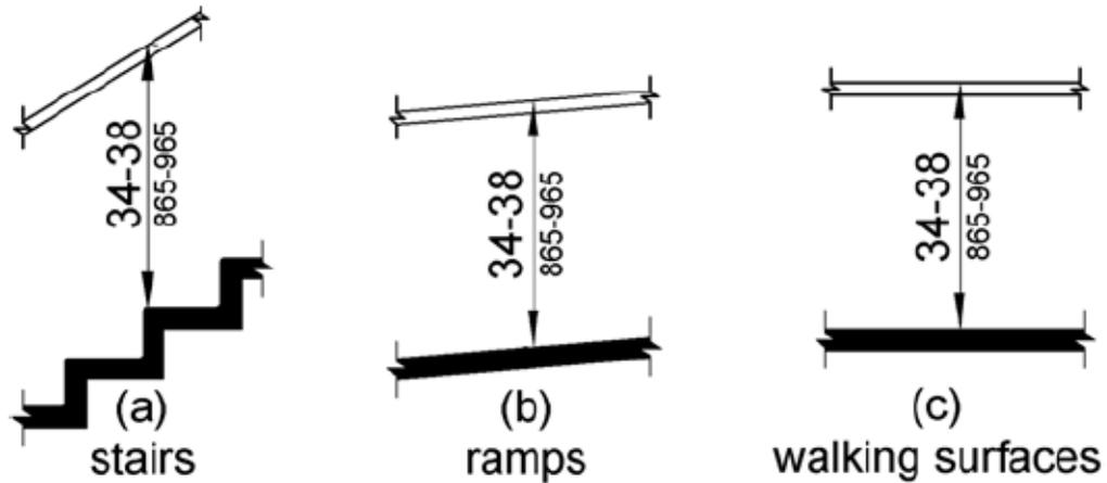
**Figure 505.4 Handrail Height**
