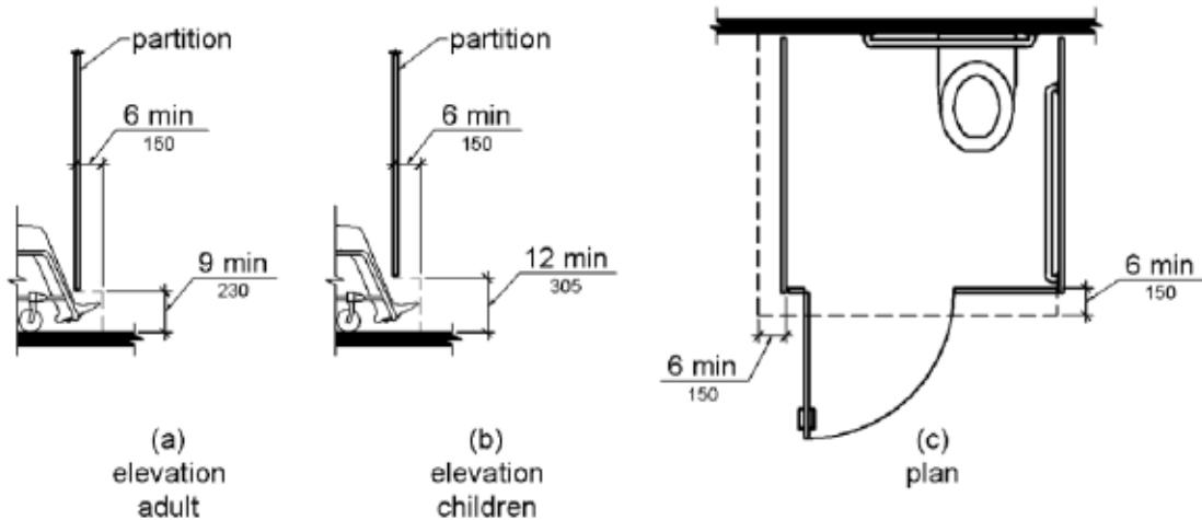
**Figure 604.8.1.4 Wheelchair Accessible Toilet Compartment Toe Clearance**
