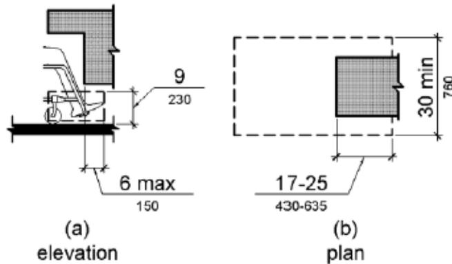
**Figure 306.2 Toe Clearance**
