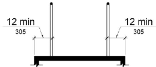
**Figure 405.9.1 Extended Floor or Ground Surface Edge Protection**
