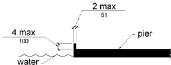
**Figure 1003.3.1 (Exception 2) Edge Protection at Boat Slips**
