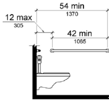
**Figure 604.5.1 Side Wall Grab Bar at Water Closets**
