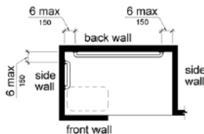
**Figure 608.3.3 Grab Bars for Alternate Roll-In Type Showers**
