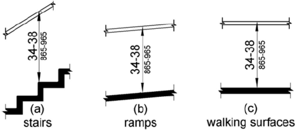
**Figure 505.4 Handrail Height**
