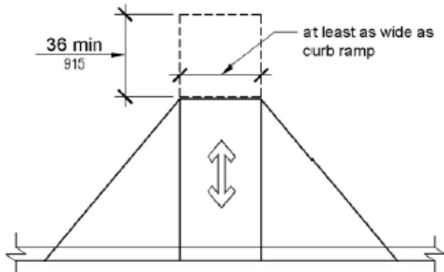
**Figure 406.4 Landings at the Top of Curb Ramps**
