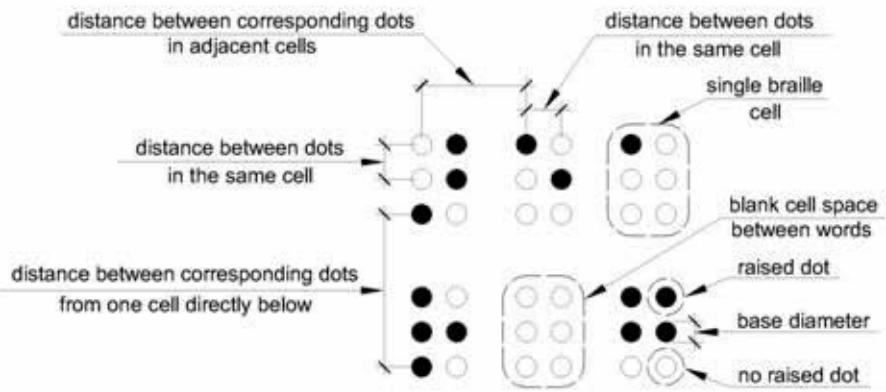
**Figure 703.3.1 Braille Measurement**
