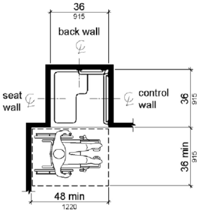
Note: inside finished dimensions measured at the center points
