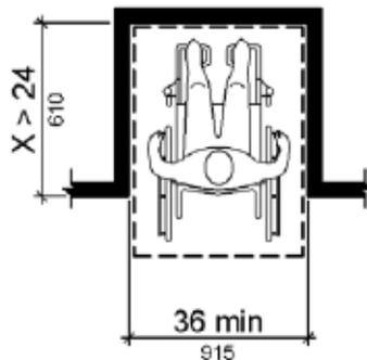
**Figure 305.7.1 Maneuvering Clearance in an Alcove, Forward Approach**
