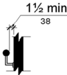
**Figure 505.5 Handrail Clearance**
