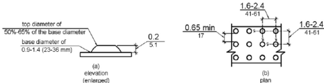
**Figure 705.1 Size and Spacing of Truncated Domes**
