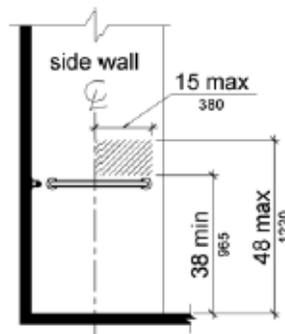
**Figure 608.5.1 Transfer Type Shower Compartment Control Location**
