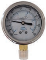
ILCG36025-4LNL. GAUGE 2-1/2" Liquid Filled, 30-0-60, 1/4" MIPT Lower Connection
