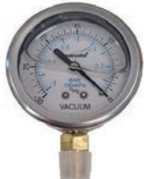
ILVG3025-4LNL GAUGE 2-1/2" Liquid Filled, 30-0, 1/4" MIPT Lower Connection
