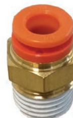
KQ2H07-35AS QUICK CONNECT FITTING Straight .250" MIPT x .250" Tubing Connection
