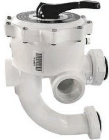
Multiport Valve for Triton (SM20-3), 7-1/2" Centerline with 2" threaded female connections.
