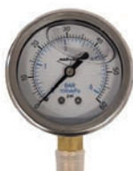
ILPG6025-4LNL. GAUGE 2-1/2" Liquid Filled, 0-60, 1/4" MIPT Lower Connection
