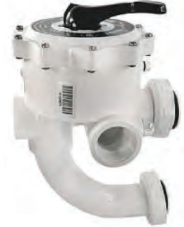
Multipoint Valve for Triton (SM20-3), 7-1/2" Centerline with 2" threaded female connections.
